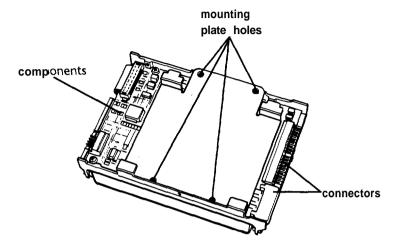
4. Locate the four screws that you removed from the 5¼-inch mounting frames and use them to secure the mounting plate to the hard disk drive.
